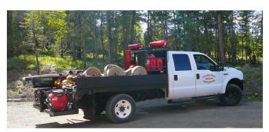
the scene faster. Last fall the fire department purchased a 2002 flatbed one ton pick-up, which we retro-fitted to a hose/pump apparatus (Water Supply #1). This will allow us to deliver more water in a shorter time frame right up to the main road and, in some cases, right to the fire scene. We would like to thank all of our members who helped to retro-fit this apparatus. It exceeds our expectations and is a huge asset for our fire protection area.
